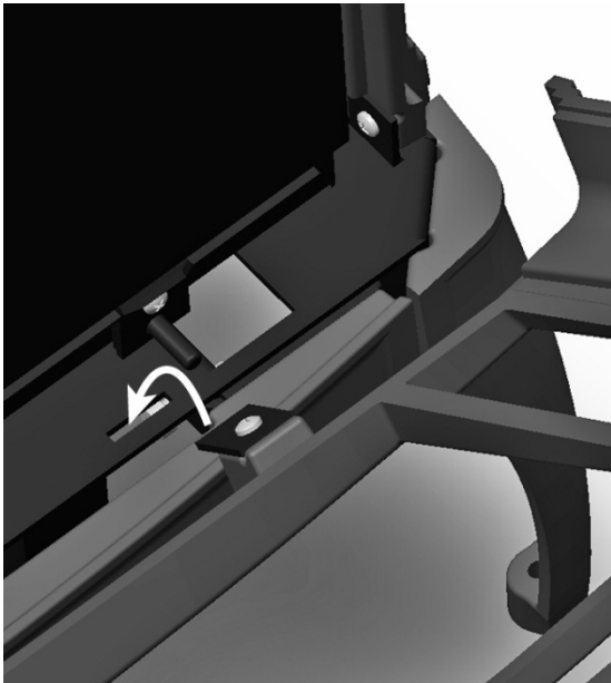
Figure 12 – Front Panel Retaining Slots
