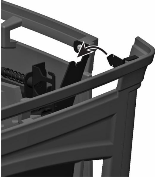
Figure 11 – Front Panel Mounting Tang Detail
