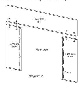
If the insert is going to sit on the hearth proceed to "Faceplate Trim Installation" (step 8) otherwise continue on to "Bottom Faceplate Installation" (step 4).
