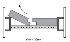
Important: push both baffle bricks so they are tight against the side walls and to the back.
