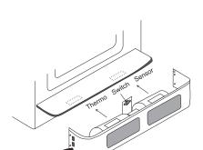
Do not turn fan ON until your insert has reached operating temperature or at least 30 minutes after starting fire.
