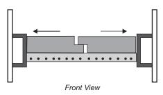
Note: When getting the chimney cleaned, remove the baffle bricks for access to the flue, then replace them when cleaning is completed.
