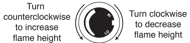
Fig. 55 Flame adjustment knob for SIT valve.
