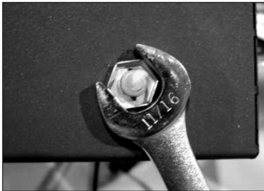
Figure 8.18 Install the speed control (rheostat). The speed control mounts to the decorative cover removed in Step 5. Insert the stem of the speed control through the hole located on the right side of the cover. Secure with the pal nut using an 11/16 in. (17.5 mm) wrench. Attach the black and white wires routed under the appliance indicated in Figure 8.13 , on page 34, to the two speed control wires. Push the speed control knob onto the stem and re-attach the decorative cover. Secure the wires up and out of the way using the zip tie provided.
