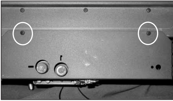
Figure 8.16 With the cast iron front of the appliance removed, remove the decorative cover located under the appliance. To remove the cover, remove the two screws on the front of the appliance that hold the cover in place. Pull the cover forward, down and out.
