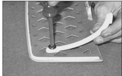
Figure 8.29 Install warming shelf bracket loosely to each warming shelf using the screw provided.
