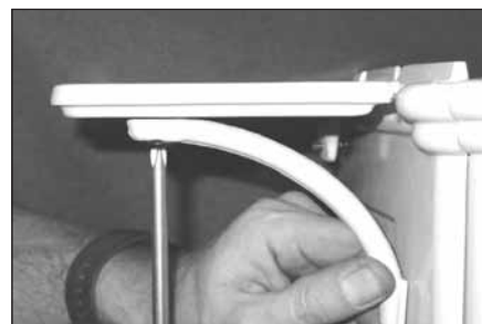
Figure 8.31 Align bracket to firebox and gently tighten the screw to hold it in place. Reassemble the appliance.
