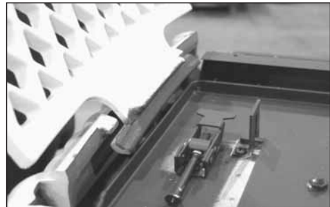
Figure 8.29 Install warming shelf bracket loosely to each warming shelf using the screw provided.
