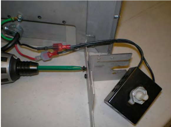
Attach Fan Control Switch Extension Bracket using [2] #6 Combo Screws as shown.
