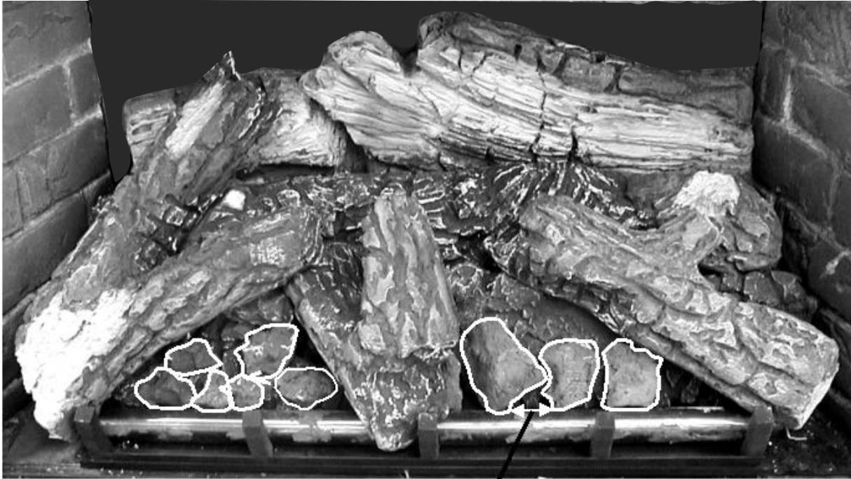
Add Large Chunk Coals behind front burner and on Logs "C" and "D" surfaces. Space Coal Chunks apart at least 1/4" where they touch the Front Burner to allow upward flow paths for Front Burner Flames.
